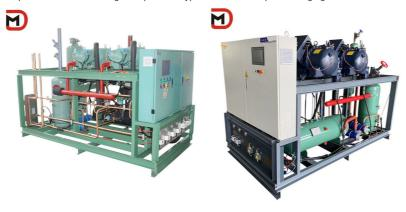
The intermediate-temperature type compressor system is designed to operate at an evaporating temperature ranging from -15°C to -30°C. The compressor motor of the intermediate-temperature type has a nominal power ranging from 50HP to 540HP. The low-temperature type compressor system is designed to operate at an evaporating temperature ranging from -35°C to -45°C. The compressor motor of the low-temperature type has a nominal power ranging from 50HP to 540HP.
