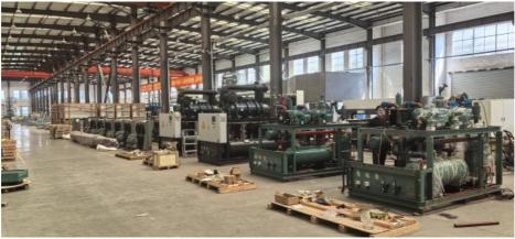
On the other hand, the intermediate-temperature type is designed for cooling systems that require an evaporating temperature range of -15°C~-30°C. The compressor motor of this type has a nominal power ranging from 50HP to 540HP. This type is ideal for applications that require moderate temperature ranges.
