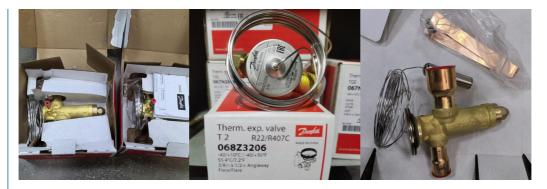
The thermostatic expansion valve regulates the flow of refrigerant liquid entering the evaporator. The flow is controlled by a thermal ball valve connected to the evaporator outlet suction line. The thermal bulb senses the evaporator heat and modulates the valve to allow refrigerant liquid entry depending on the refrigeration load.
