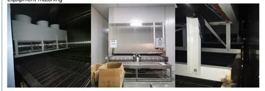
The quick freezing tunnel is used to transport products from the inlet to the outlet through a conveyor belt, where multiple air-cooled evaporators supply air to the product to quickly cool the product at room temperature in a short period of time, achieving the effect of quick freezing.
