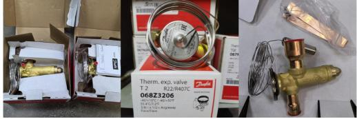
Thermostatic expansion valve regulates the flow of liquid refrigerant entering the evaporator. The flow is controlled by a thermal ball valve attached to the evaporator outlet suction pipe. Thermostatic ball sensing evaporator heating and regulating valve
