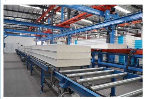
We adopt OMS high-pressure pentane foaming system and Siemens intelligent production control technology to realize "fluorine-free green production" and "fully automated intelligent production". This production mode not only meets the requirements of environmental protection and reduces the damage to the ozone layer, but also greatly improves the production efficiency and product quality.
